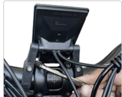
Insert the handlebar into the adjustment position, fasten the buckle, and tighten the screw.
