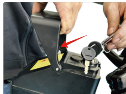
Lift the battery upward.
