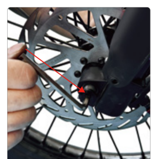
Tighten the nuts to complete the installation.
