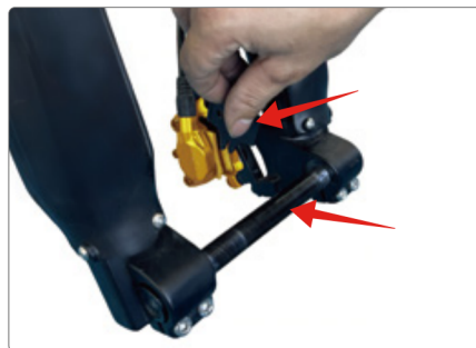
First remove the quick-release lever, then extract the spacer.
