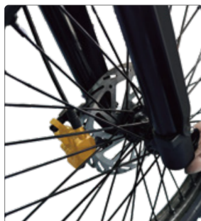
Putting the tyre into the fork slot
