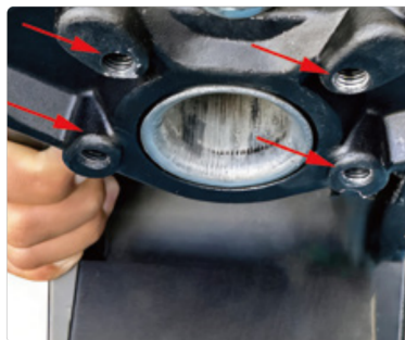
Tighten each screw into its corresponding hole.
