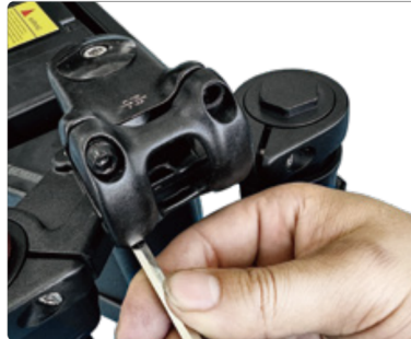
Then unscrew the four screws on the buckle.
