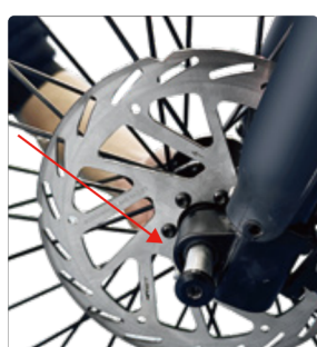
Insertion of quick release lever
