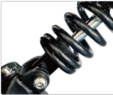
Align the rear shock absorber with the mounting holes on the frame.
