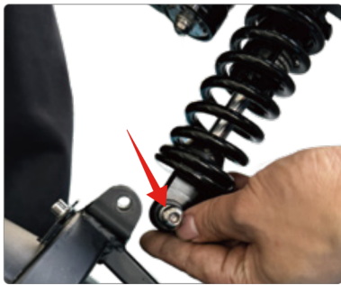
Install the screws at the shock absorber.
