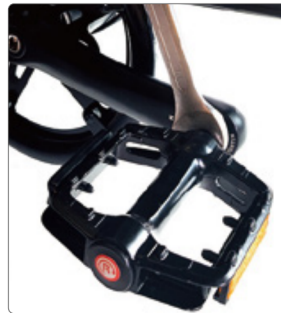
Tighten the left pedal "L" counter clockwise
