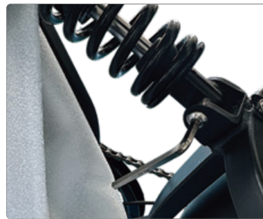
Tighten all fixing screws in sequence.
